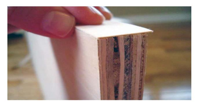
5. With your edgebanding in position, apply the iron to melt the glue.
