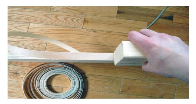
Press firmly and slide the block back and forth over the section that you ironed making sure that the veneer fully adheres to the plywood. This pressure is necessary to ensure a firm strong bond with the glue line and your edge. A good bond will prevent you from pulling the edgebanding up off the plywood in any place along the edge. You don't want the edgebanding to delaminate once your project has been completed.
