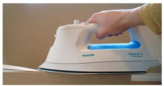
"Pressing" firmly is preferred rather than an "ironing" technique. Just hold your iron in one spot for about 20 seconds. It will take time for the hot iron to soften the glue line enough
